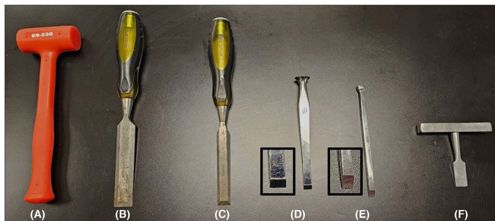
FIGURE 8 Hammer and chisels. (A) Mallet. (B) Wide wood chisel. (C) Narrow wood chisel. (D) Wide bone chisel. (E) narrow bone chisel. (F) T-chisel.
