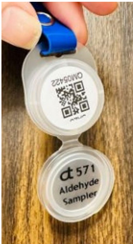
FIGURE 1 Representative picture of a wearable air quality monitoring device, which may be sent to the manufacturer for analysis.
